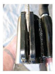
Lube the spindle with automotive grease.
