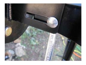
Insert grease fitting and thread in using a 5/16" wrench. Install snap ring.
