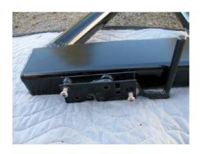
Install the detent stud with the supplied spring on it. Lube the detent before installing.
