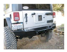
Tighten the bolts into the side of frame using a 16mm socket.
