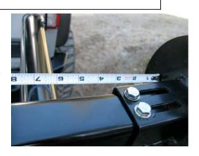
Insert two 5/16"x3/4" carriage bolts, use flat washer and 5/16" nylock nuts. Tighten with ½" wrench.
