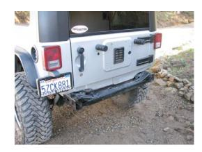
Retain the stock bolts that attached the bumper to the sides of the frame.
