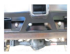
Adjust bumper making sure the top is running parallel with the ground. Stand back and make sure it is aligned with the back of the vehicle.
