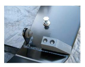
Lift rear bumper into place and set over onto the frame horns.
