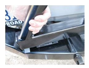
With the tire carrier in the closed position insert the 2@ 5/16" x 1 1/4" bolts thread on the c-nuts(self locking). Tighten the nuts until snug. Do not over tighten, the clamp sleeve should not touch it self. Test tightness by opening the tire carrier carefully. The tire carrier should not droop to hit the bumper. Work tire carrier back and forth and readjust if necessary.
