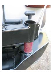
Work the tire carrier back and forth until the tire carrier is all the way down onto the spindle.
