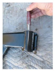
Thread on the 7/16" nut and the tee handle. Tighten the nut against the tee handle to lock the tee handle in place.
