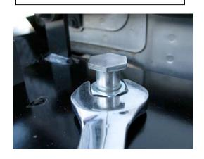
Insert the 2 @  $\frac{1}{2}$ " x 1  $\frac{1}{2}$ " bolts with a flat washer and nut locking into position. Hand tighten.
